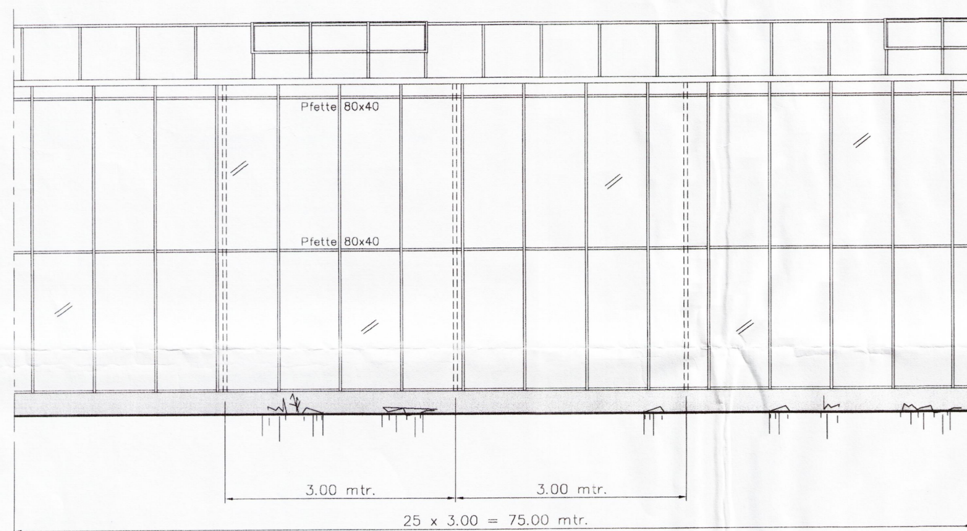
Detail view sidewall scale 1 : 50
